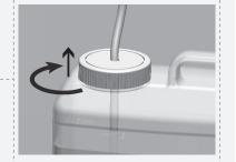
Place the cover back and screw it closed, making sure the hose extends to the bottom of the soap bottle.
