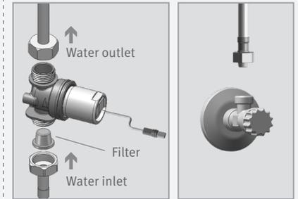
Note: Make sure that the filter is assembled between the housing of the solenoid valve and the adapter.
