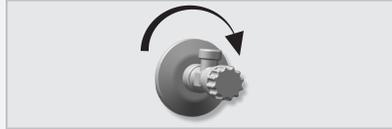
2 Remove the hexagonal nut, the disk and the gasket. Do not remove the O-ring from the base of the faucet.
