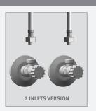
MAKE SURE THAT THE FILTERS ARE INSTALLED BETWEEN THE FLEXIBLE PIPE AND THE SHUT OFF VALVE/ANGLE VALVE (NOT SUPPLIED).
