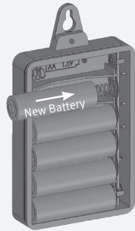
4. Replace the used batteries with a new 6 X 1.5V batteries (Lithium battery is recommended).
